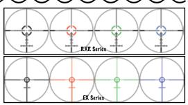
PRESMA riflescopes can be used in either the standard or the illuminated state. When not illuminated, the reticle performs the same as the reticle in a standard non-illuminated PRESMA scope. When the illumination is activated, portions of the reticle will illuminate to provide better contrast in poorly lighted conditions between the target and the precise position of the aiming point. The scope will remember the last settings used.
